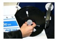
2) Place spool on spindle and tighten Knurled Nut snugly onto the spindle to secure spool.
