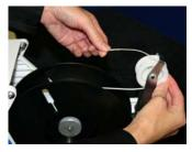
3) Feed tie material under small roller on brake arm, then over top of roller and pull towards machine.
