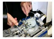
5) Pull the Idler Wheel out using lever and guide material into the Pinion Support Channel.
