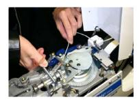
5) Pull the Idler Wheel out, using lever and guide material into the Pinion Support Channel.
