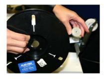
Unscrew Knurled Nut, then place spool of tie material in right hand with label facing palm.
