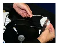
Feed tie material under small roller on brake arm, then over top of roller and pull towards machine.
