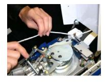
4) Feed material through the Pin on Brake Arm and pull approx 4 inches.
