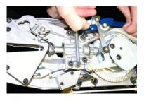
6) Continue slowly inserting the ribbon into Pinion Support Channel until the ribbon appears just beyond the cutter. Make sure that the ribbon is under the lip of the white plastic ribbon guide.
