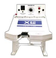
The HEAVY-DUTY XL2 model features an extra wide opening specifically designed for tying products from 1/2" to 2" in diameter. With up to 40 ties per minute, the ever adaptable XL2 seamlessly handles bag-in-box and flow-through packaging operations with ease.
